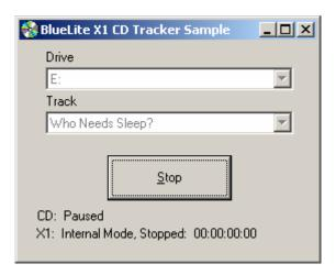
At this point, selecting Play or Record on the X1's Event List Window will cause the CD to seek to the equivalent time and begin playing. For example, starting at an X1 time of 00:00:00:00 will begin playing the track from its start. An X1 time of 00:00:30:00 will start the CD 30 seconds into the track, and etc.
